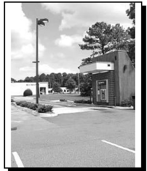
This ATM is well lit and is located for visibility from the main parking area and the public street.
