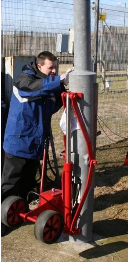
Demonstrating a one-man column lowering tool
