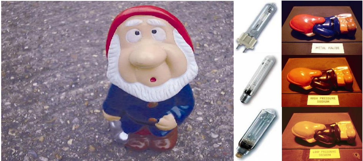
Effect of Colour Rendering with different lamps
