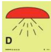
6028 Space protected by drenching
