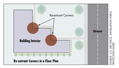
Figure 3-2 Re-entrant corners in a floor plan
