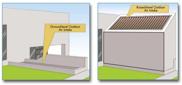
Figure 3-10 Another example of protecting outdoor air intakes
