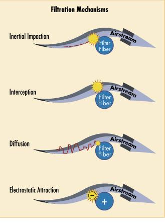
Figure 5-3 Four primary filter collection mechanisms
