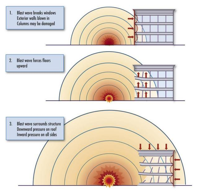
Figure 4-4 Blast pressure effects on a structure
