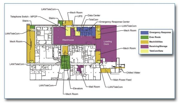
Figure 1-10 Non-redundant critical functions collocated near loading dock
