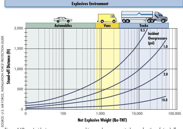
Figure 4-10 Incident overpressure measured in pounds per square inch, as a function of stand-off distance and net explosive weight (pounds-TNT)
