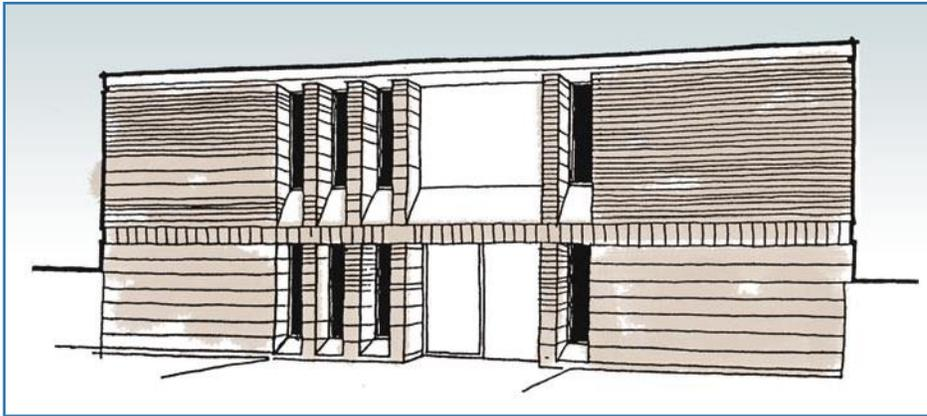
Figure 3-6 Narrow and recessed windows with sloped sills
