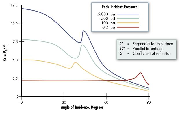
Figure 4-2 Reflected pressure coefficient vs. angle of incidence
