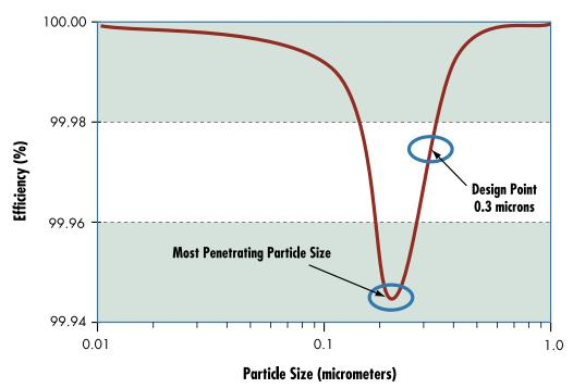
Figure 5-7 Typical performance of a HEPA 99.97%
