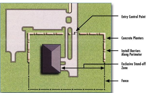
Figure 2-11 Application of perimeter barrier elements
